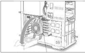
Lowering the auxiliary fan (retaining clip on 8500)
